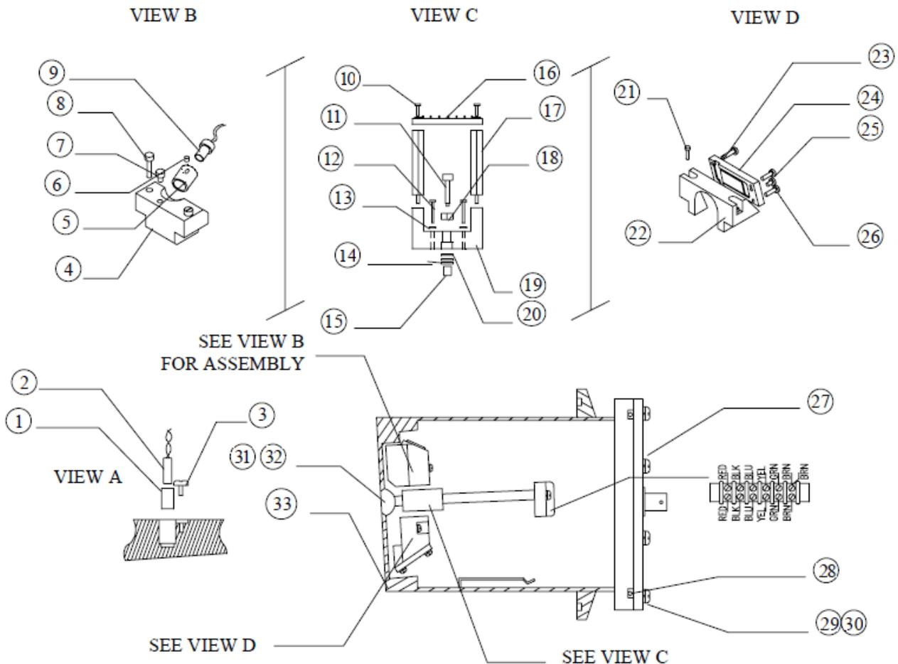
The drawing demonstrates our probe with a 4" tri-clamp flange and no prism wash. Any Industrial flange is available if sanitary fittings are not required, including ANSI, JIS, DIN/PN. These are represented by a dash after the part number; contact an LSC sales representative for a part number specific to your application before ordering.
